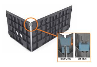
**STEP 3** – Connect the remaining short wall to the other end of the long wall with two fastclips as per steps 1 & 2.
