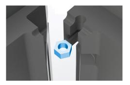
**STEP 2** – Connect one short wall to one long wall vertically with two fastclips at the connection angle.
